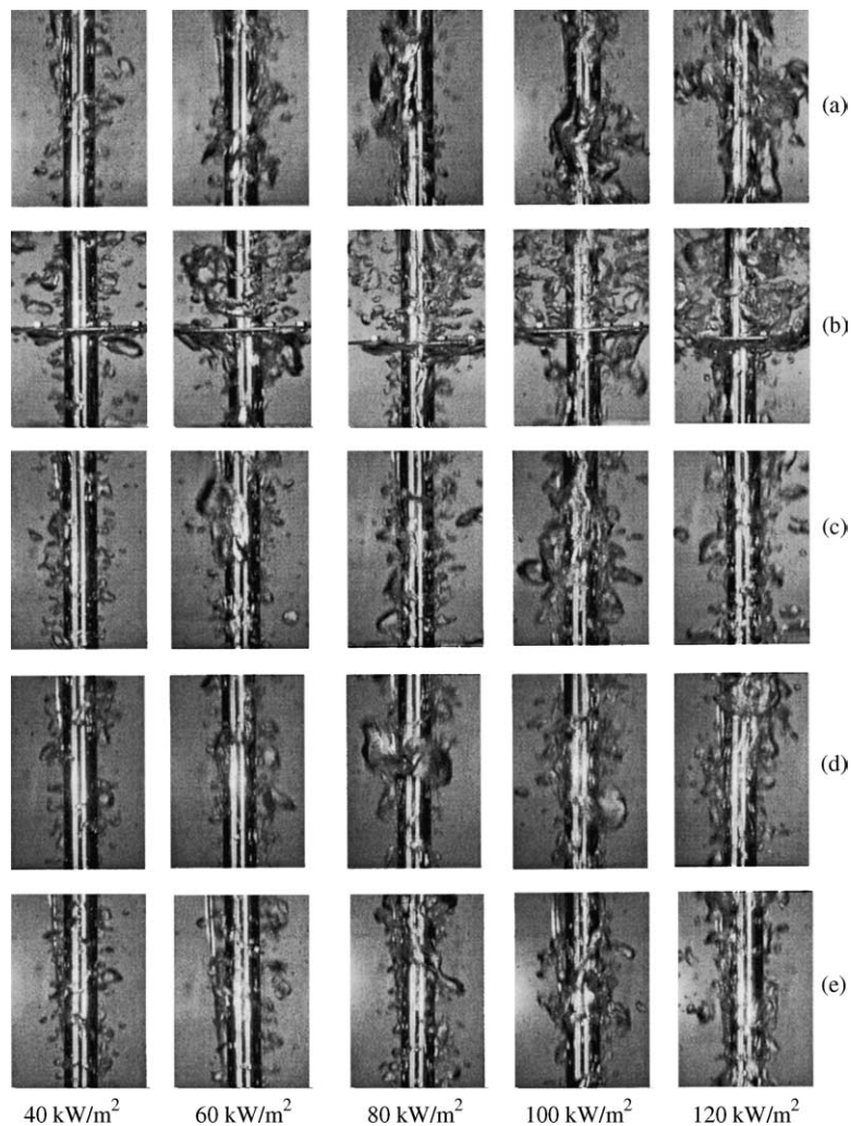
Fig. 6. Photos of pool boiling as the location of the flow disturbing plate ( D_0 = 79.1 mm) changes. (a) Single tube, (b) LP = 460 mm, (c) LP = 360 mm, (d) LP = 260 mm and (e) LP = 160 mm.
